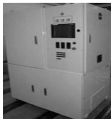
Photo 1. Appearance of the ammonia gas removal device
