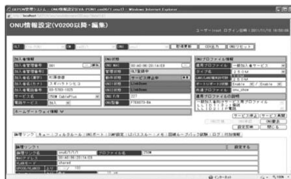
Photo 10. GE-PON Management System Screen Sample (ONU setting)
