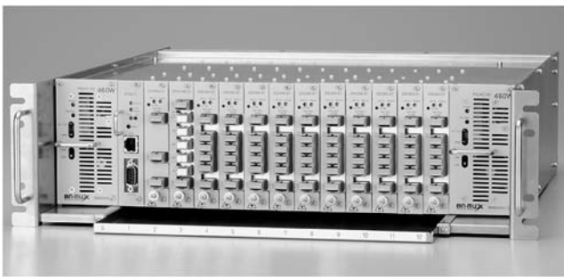
Photo 1. Integrated Headend Equipment (BN8200C Series)
