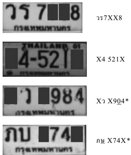
Fig. 4. Examples of the result of character recognition. The results with asterisk (*) are recognition failure, and characters with under bar are misrecognized.
