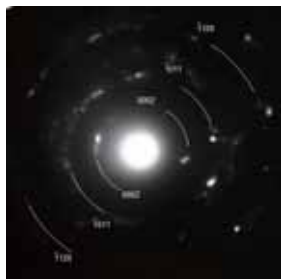
Fig. 5. A TEM photograph and electron diffraction pattern of the edge of the BG-CNS in Photo 4
