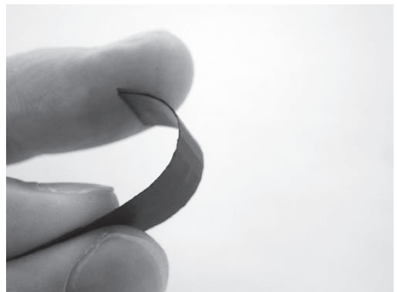
Photo 2. Antenna section incorporating Sumitomo Electric's FPC
