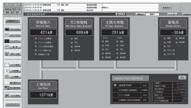
Fig. 5. Operation control main window
