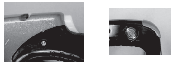
photo 3. Exposed metal parts at edges (enlarged view of the circled part O shown in Fig. 5)
