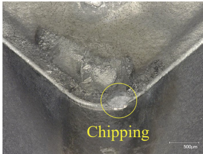
Photo 1. Example of cutting tool edge damaged in high-efficiency machining
