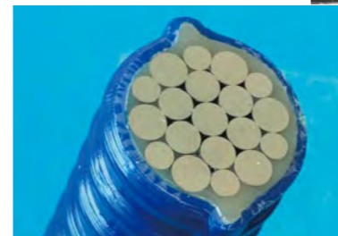
Pre-grouted prestressing steel strand
