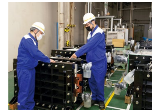
Closely check completed cell stacks
