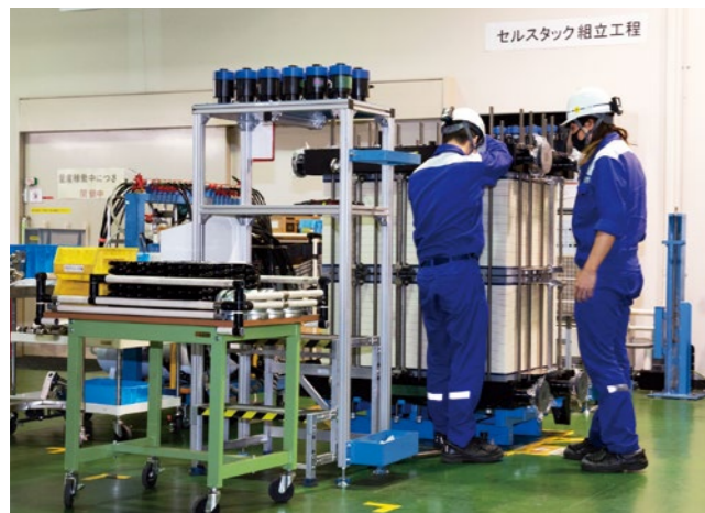
Assembly process for cell stacks
