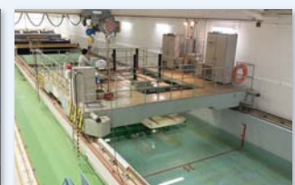
Study to understand hydro dynamical phenomena related to vessels in an experimental tank
