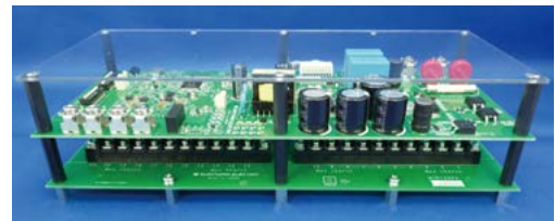
PLC string monitoring unit for 1,500 V DC plants
