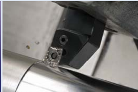
"T1500A" realizing smoother finished surface by fine-grain-size control.
