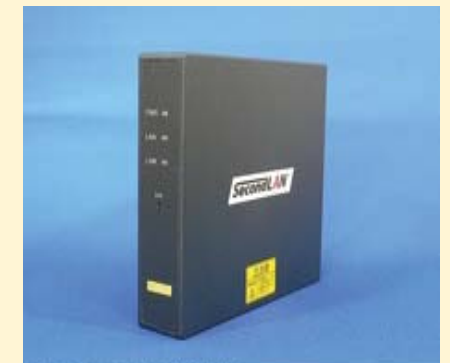
"MC3000" modems to create high-speed network by using existing community coaxial TV cable in building. (Nov. 2010).
