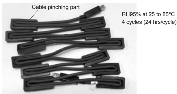
Photo 2. Test sample for a complex test of cable pinching and temperature and humidity changes
