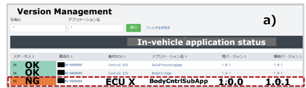
Fig. 9. The system detects that the version of the BodyCtrlSubApp, an application installed on the ECU X, is not the latest version (area enclosed by dashed lines in the figure). The administrator clicks on the area in question to view the details.
