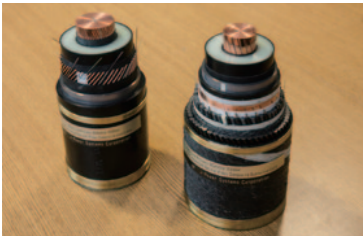
400 kV DC XLPE insulated cable samples: land cable (left) and submarine cable (right)
