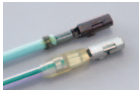
Corroded terminal (upper) and corrosion-free terminal protected by a mold (lower)
