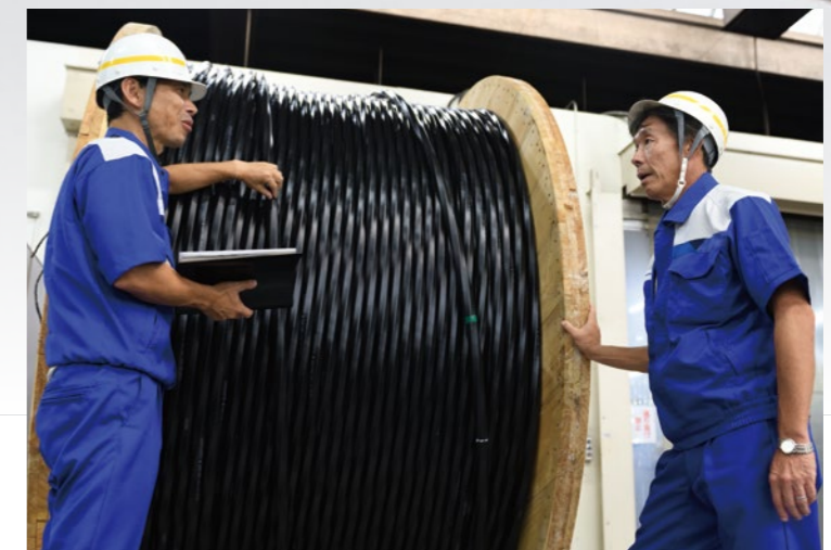
3456-fiber-count optical cable awaiting shipment (left: Takehiko Okada, General Manager of the Cable Manufacturing Dept., right: Tsuguo Amano, General Manager of the Engineering Dept.)
