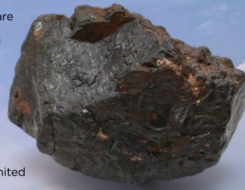
Tungsten ore. The percentage of tungsten contained in the ore is less than 1%.
