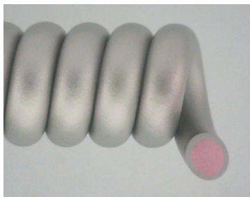
Photo 2. Processing example of SUS-covered Cu wire as a spring
