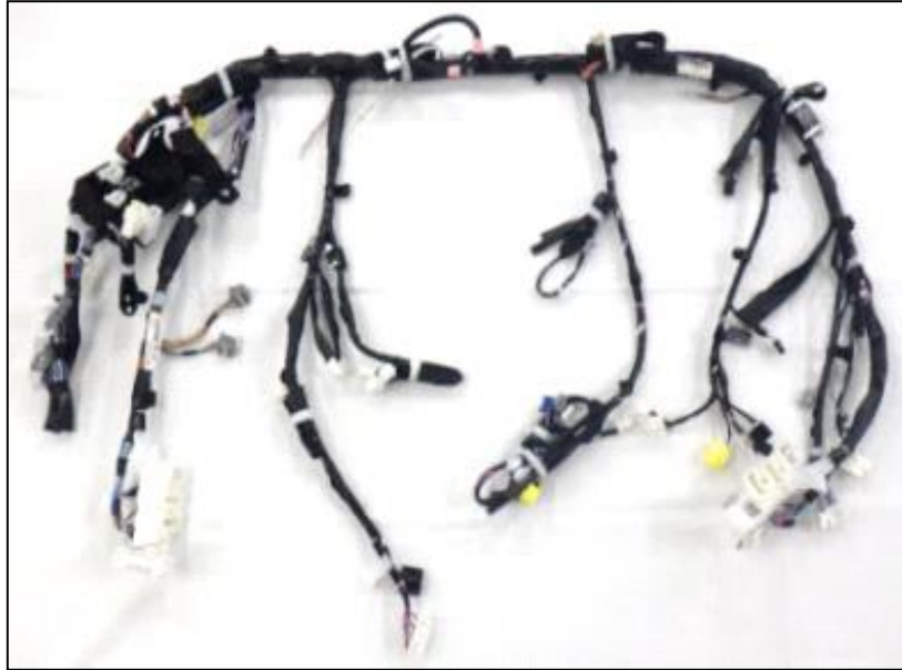
Existing integrated wiring harness
