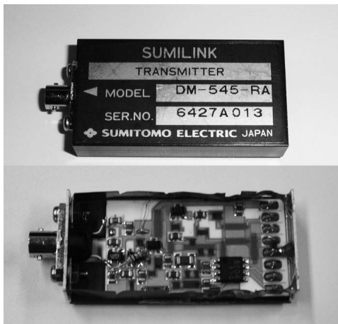
Photo 4. Optical Data Link for FDDI (Upper) , Receiver (Lower) Receiver Front-end by GaAs-FET, SOP-IC is Custom-designed IC
