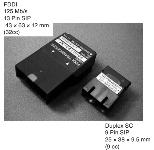
Photo 5. Comparison of FDDI and Duplex SC ODL
