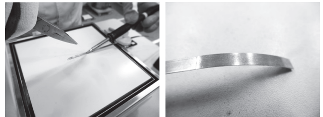
Photos 1. Peeling of the reinforcing material and the wire from which one reinforcing material is peeled off
