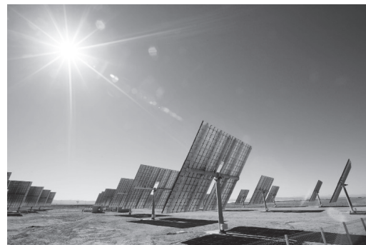
Photo 4. CPV System Tracks the Sun Precisely
