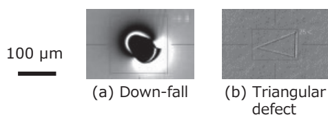
Fig. 1. SiC epitaxial defects
