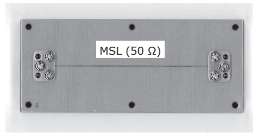
Fig. 3. MSL board for transmission characteristics evaluation (Sumitomo Electric's fluoro-resin substrate)
