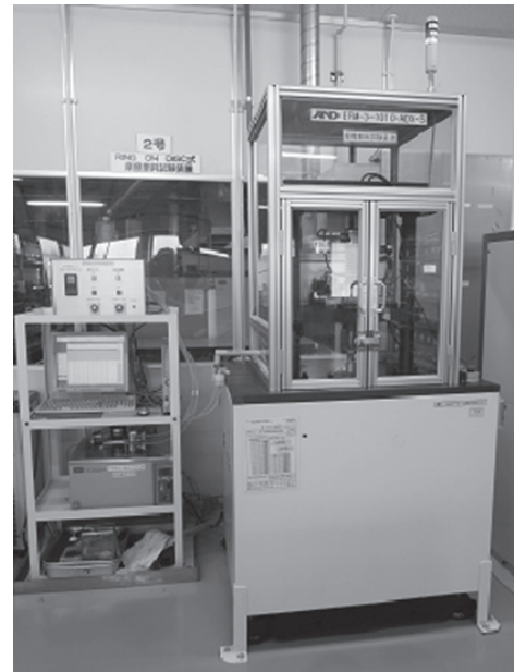
Photo 2. Ring-on-disk friction and wear test equipment
