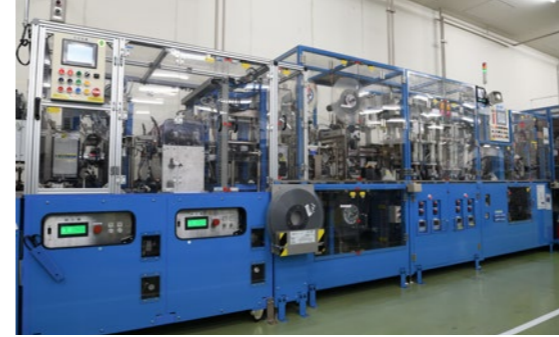
Tab-lead manufacturing system of Sumitomo Electric Wire, Inc.
