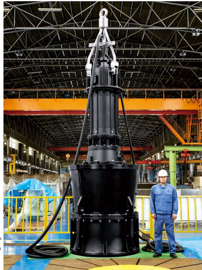
Submersible axial-flow column pump of Japan's largest-class diameter using S-FREE™ traveling cables (Photo courtesy of Tsurumi Manufacturing Co., Ltd.)
