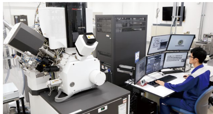
Focused Ion Beam Scanning Electron Microscope (FIB-SEM) is the main equipment for cross section preparation and observation.
