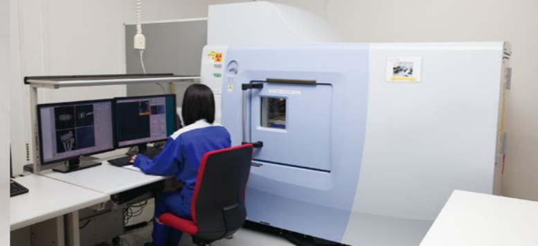
A micro-focus X-ray CT scanner uses X-rays to perform nondestructive three-dimensional observation of the internal structure of a specimen.
