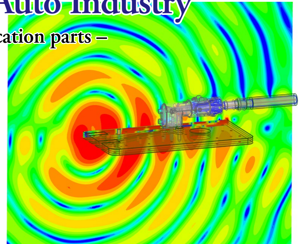
This electromagnetic noise radiation chart based on high-frequency CAE shows the strength of waves during electromagnetic radiation at the connector (red: strong). The waves propagate in varying intensity.
