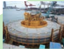
Extra high voltage DC cable
