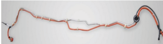
Photo 9. Example of an under-floor wiring harness
